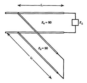
25. For each of the following load impedances in the doublestub tuning transmission line system shown, find stub lengths  $l_1$  and  $l_2$  to match the load to the line.
