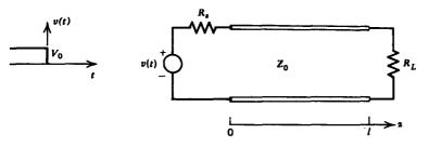
(b) Find the voltage at the z = l end as a function of time. (Hint: Use difference equations.)
