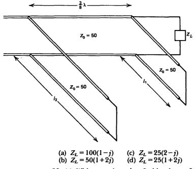
26. (a) Without using the Smith chart, find the input impedance  $Z_{in}$  at  $z = -l = -\lambda/4$  for each of the loads shown. (b) What is the input current i(z = -l, t) for each of the loads?
