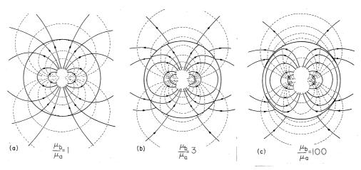
Fig. 9.6.2 Magnetic potential and lines of field intensity in and around the magnetizable sphere of Fig. 9.6.1. (a) With the ratio of permeabilities equal to 1, the dipole field extends into the surrounding free space region without modification. (b) With  $\mu_b/\mu_a = 3$ , field lines tend to be more confined to the sphere. (c) With  $\mu_b/\mu_a = 100$ , the field lines (and hence the flux lines) tend to remain inside the sphere.
