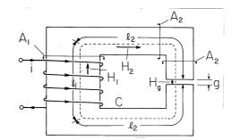
Fig. 9.7.3 Cross-section of magnetic circuit used to produce a magnetic field intensity  $H_g$  in an air gap.
