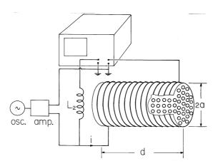
Fig. 9.5.4 Experiment to measure the decrease of inductance that results when the artificial diamagnetic array of Fig. 9.5.2b is inserted into a solenoid.
