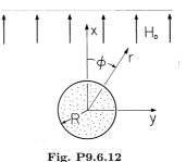
**9.6.13** The spherical coil of Example 9.6.1 is wound around a sphere of material having the B - H curve shown in Fig. P9.6.11. Assume that i = 800 A,
