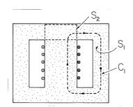
**Fig. 9.7.2** Cross-section of highly permeable core showing contour  $C_1$  spanned by surface  $S_1$ , used with Ampére's integral law, and closed surface  $S_2$ , used with the integral flux continuity law.
