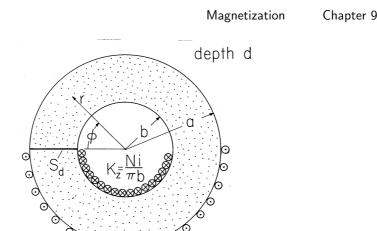
**Fig. 9.7.5** Magnetic circuit consisting of a core having the shape of a circular cylindrical annulus with an *N*-turn winding wrapped around half of its circumferential length. The length of the system into the paper is very long compared to the outer radius *a*.
