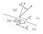
Fig. 9.6.3 Graphical representation of the relations between components of H at an interface between a medium of permeability  $\mu_a$  and a material having permeability  $\mu_b$ .
