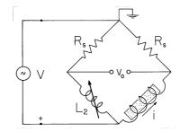
Fig. 9.5.5 Bridge used to measure the change in inductance in the experiment of Fig. 9.5.4.
