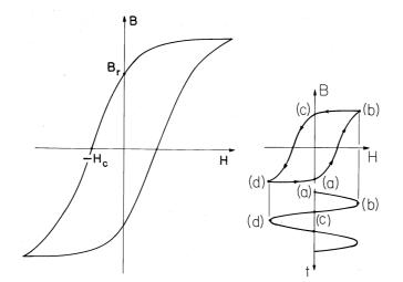
**Fig. 9.4.6** Magnetization characteristic for material showing hysteresis with typical values of  $B_r$  and  $H_c$  given in Table 9.4.2. The curve is obtained after many cycles of sinusoidal excitation in apparatus such as that of Fig. 9.4.3. The trajectory is traced out in response to a sinusoidal current, as shown by the inset.
