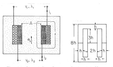
Fig. 9.7.7 In a typical transformer, coupling is optimized by wrapping the primary and secondary on the same core. The inset shows how full use is made of the magnetizable material in the core manufacture.
