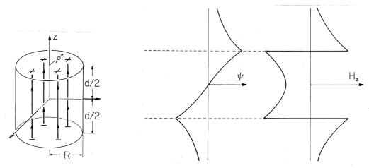
**Fig. 9.3.1** (a) Cylinder of circular cross-section uniformly magnetized in the direction of its axis. (b) Axial distribution of scalar magnetic potential and (c) axial magnetic field intensity. For these distributions, the cylinder length is assumed to be equal to its diameter.
