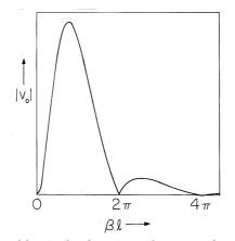
Fig. 9.3.4 Magnitude of sensing coil output voltage as a function of  $\beta l = 2\pi l/\Lambda$ , where  $\Lambda$  is the wavelength of the magnetization. If the magnetization is produced by a fixed coil driven at the angular frequency  $\omega$ , the horizontal axis, which is then  $\omega l/U$ , is proportional to the recording frequency.
