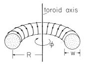
Fig. 9.4.1 Toroidal coil with donut-shaped magnetizable core.
