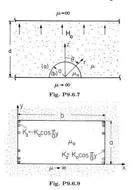
**9.6.9**<sup>\*</sup> A cylindrical region of free space of rectangular cross-section is surrounded by infinitely permeable material, as shown in Fig. P9.6.9. Surface currents are imposed by means of windings in the planes x = 0 and x = b. Show that
