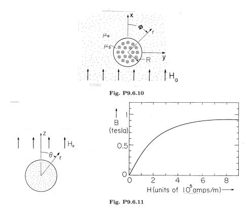
(a) Assume that the magnetization density is  $\mathbf{M} = M\mathbf{i}_{\mathbf{z}}$ , where M is a constant to be determined, and show that the magnetic field intensity inside the sphere is uniform, z directed, and of magnitude  $H = H_o - M/3$ , and hence that the magnetic flux density, B, in the sphere is related to the magnitude of the magnetic field intensity H by
