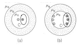
**Fig. 9.6.5** (a) With coil in the low permeability region, the contour encircling the current must pass through low permeability material. (b) With coil on the surface between regions, contours encircling current must still leave highly permeable region.
