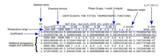
Figure 1: How to read NASA thermodynamic coefficients tables.
