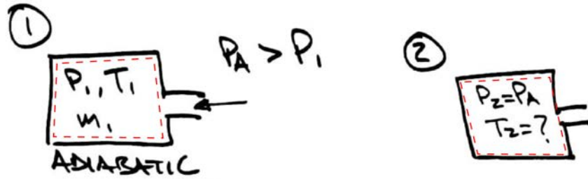
Figure 5.8: Example where an adiabatic container is initially at some pressure P_1 < P_a and then opens to allow ambient air to rush in.
