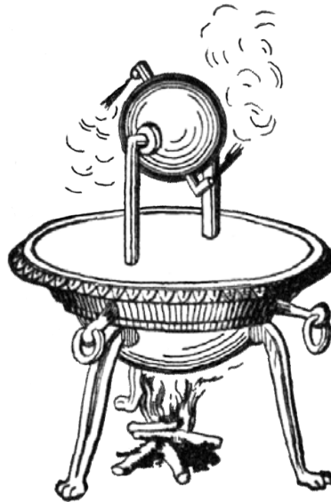
Figure 4.1: An aeolipile, which is considered to be the first engineered coupled thermodynamic system that converts thermal to mechanical energy. Virtruvius first described this device in the first century BCE. This image is in the public domain.
