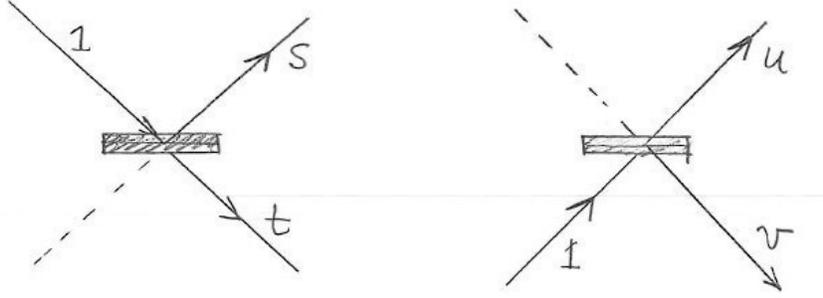
Figure 3: Left: A photon incident from the top;  $s$  and  $t$  are the reflected and transmitted amplitudes, respectively. Right: A photon incident from the bottom;  $v$  and  $u$  are the reflected and transmitted amplitudes, respectively.
