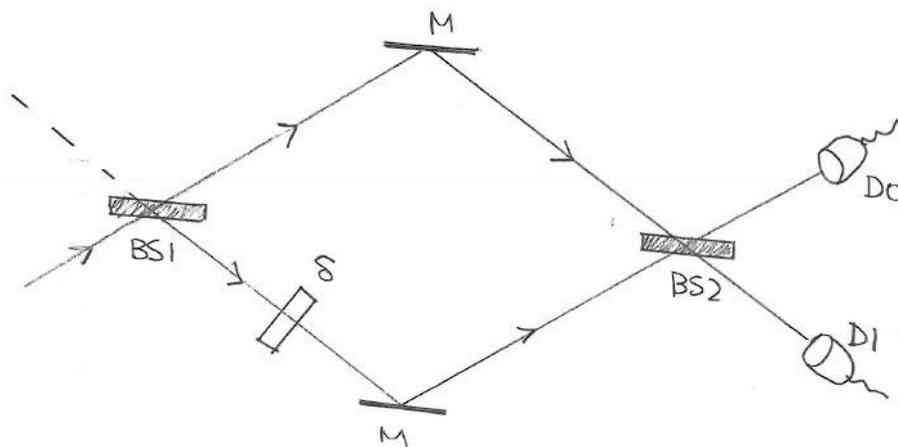
Figure 1: The Mach-Zehnder Interferometer
