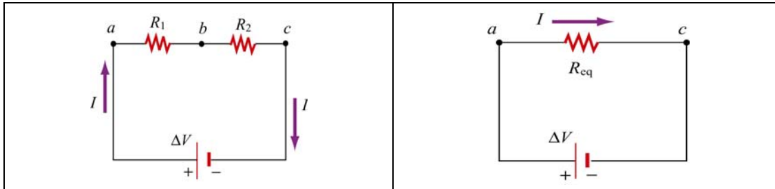
Figure 7.3.1 (a) Resistors in series. (b) Equivalent circuit.
