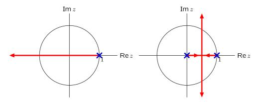
Fastest response without delay: single pole at z = 0.
