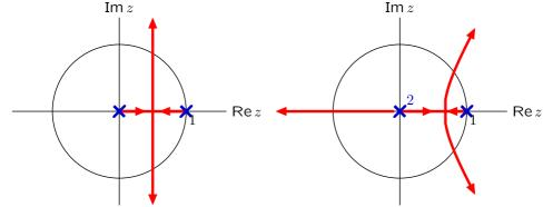
Fastest response with delay: double pole at  $z = \frac{1}{2}$ .
