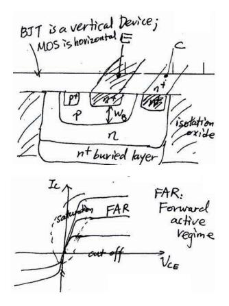
In analogy to MOSFET small current  $I_{\rm B}$  or voltage  $V_{\rm BE},$  controls large current  $I_{\rm c}$
