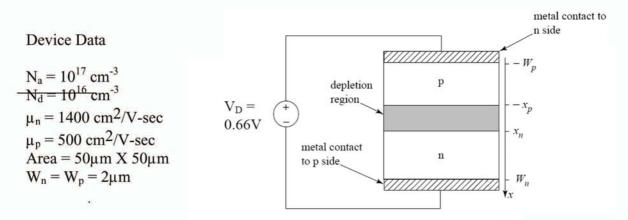
a) Calculate the total depletion region width,  $x_{D}$ , for this forward biased diode.
