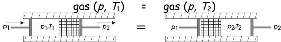
$$w = p_1 V_1 - p_2 V_2 \Rightarrow \Delta U = q + w = p_1 V_1 - p_2 V_2 = -\Delta(pV)$$
