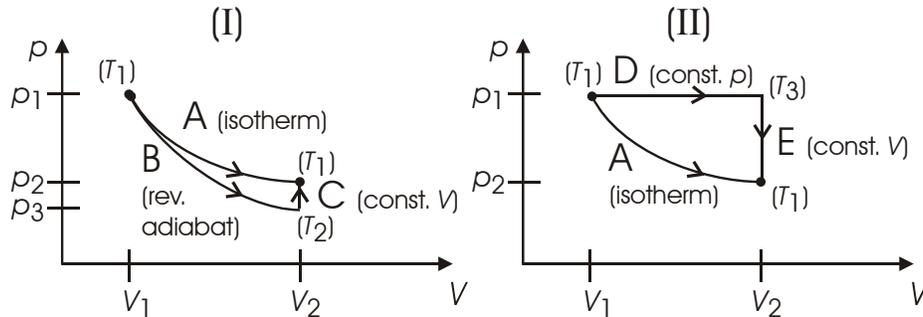
$$[A] \quad 1 \text{ mol gas } (p_1, V_1, T_1) \stackrel{\text{const. } T}{=} 1 \text{ mol gas } (p_2, V_2, T_1)$$
