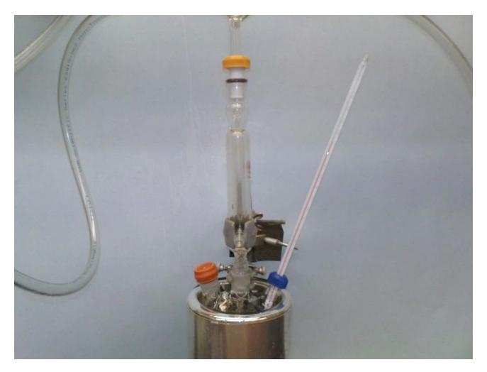
Figure 3. Set up for the in situ generation of the CAB catalyst and Diels-Alder reaction.
