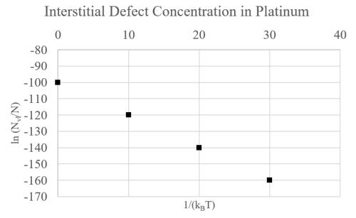
i) Estimate the formation energy (in J) of an interstitial defect from the plot. How does this compare to the vacancy formation energy in Pt, which was given above as 0.96 eV? *Hint*: assume that interstitial defect concentration follows an Arrhenius relationship. (5 points)
