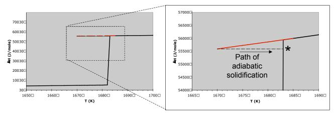
The plot is constructed by determining the enthalpy at each point using the constant pressure heat capacity. At 1500K, the silicon is in the solid state:
