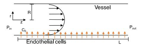
Further assume that the vessel flow is fully developed throughout the entire length and is driven by a pressure drop  $\Delta P$  across a characteristic length L. At z = 0 there is initially no TNF $\alpha$ diffused into the vessel.
