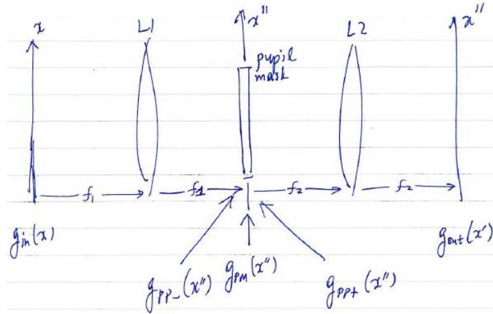
$$g_{pp-}(x'', y'') = \frac{e^{i2\pi 2f_1/\lambda}}{i\lambda f_1} G_{in} \left( \frac{x''}{\lambda f_1}, \frac{y''}{\lambda f_1} \right) \quad [\text{Fourier transform property of } L_1]$$
