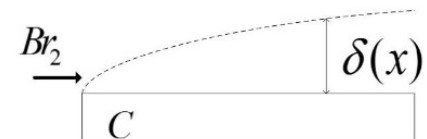
Figure 8: Flow Battery with a depletion layer of Bromine at the cathode surface
