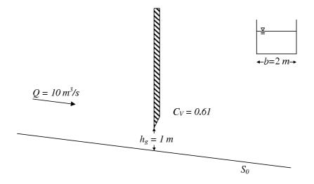
Figure 1: Flow under a gate in Problems 1-3.
