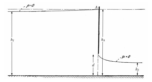
Figure 3: Sluice gate in Problem 3.
