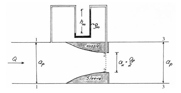
Figure 5: Pipe with nozzle-sleeve in Problem 6.
